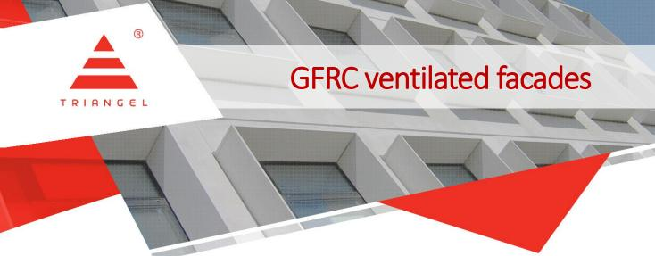
Glass Fiber Reinforced Concrete is composite material based on concrete. GFRC is made of white cement and crushed dolomite reinforced with Glass Fiber. Thanks to this combination is achieved especial technical characteristic such as: hardness, strength, durability, shapeability, fire resistance and others.
